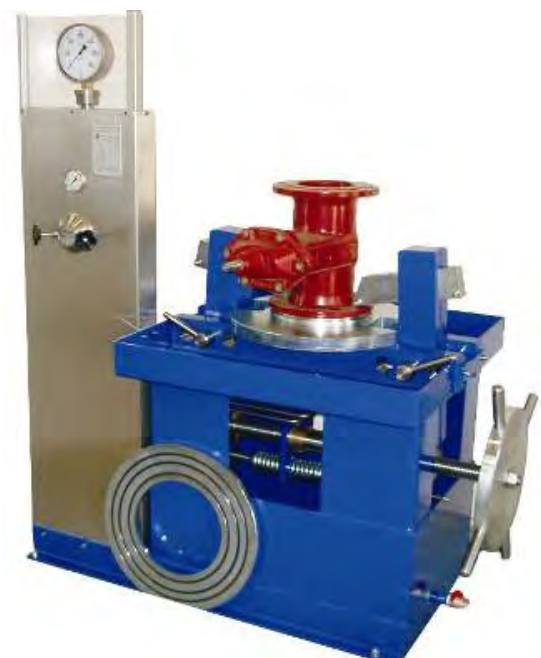
Test bench for Safety Relief Valve & Manual Valve
