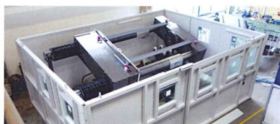
Safety enclosure with safety interlocking device
