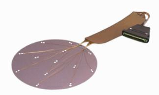
The Instrumented Wafer (Thermocouples, Bonded Wafer or RTDs) finds application in semiconductor processing equipment where knowing and controlling the temperature at the surface of a wafer is critical.
