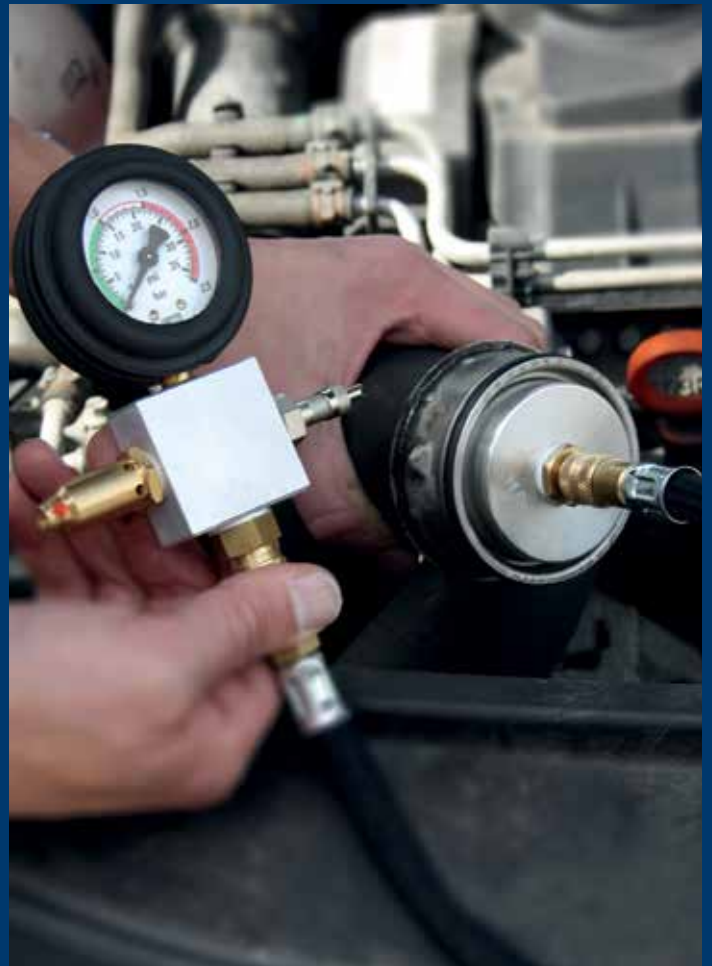
Tightness test of the cold air intake system with the MLPS.
