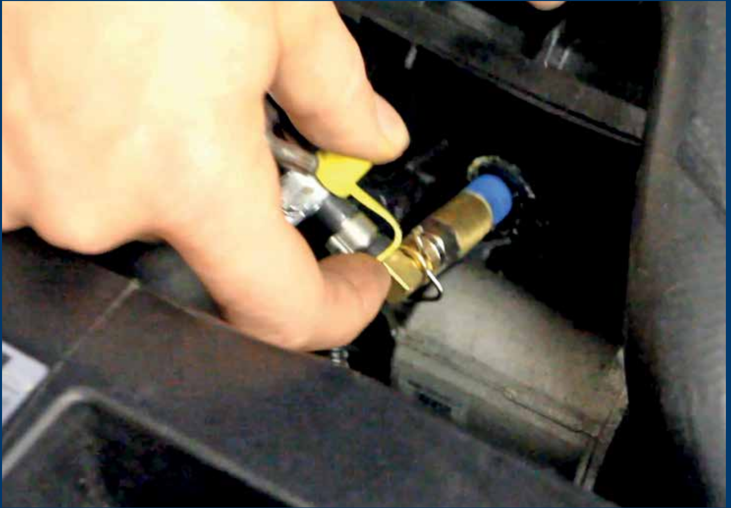
Cleaning the air intake valve with the device EVR 01.
