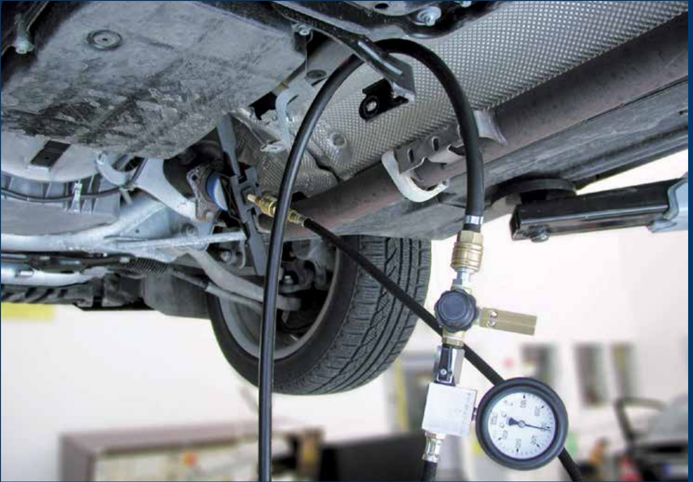
Leak test at the exhaust system with the ADP 01.
