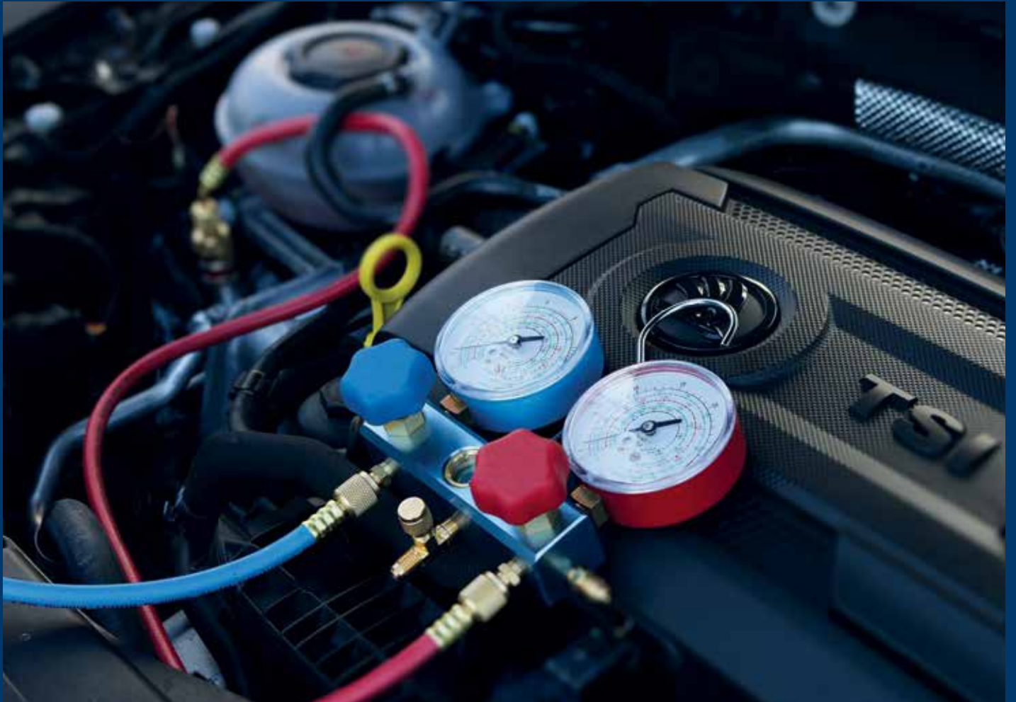
2 way manifold test kit for service and diagnosis of the air-conditioning system.
