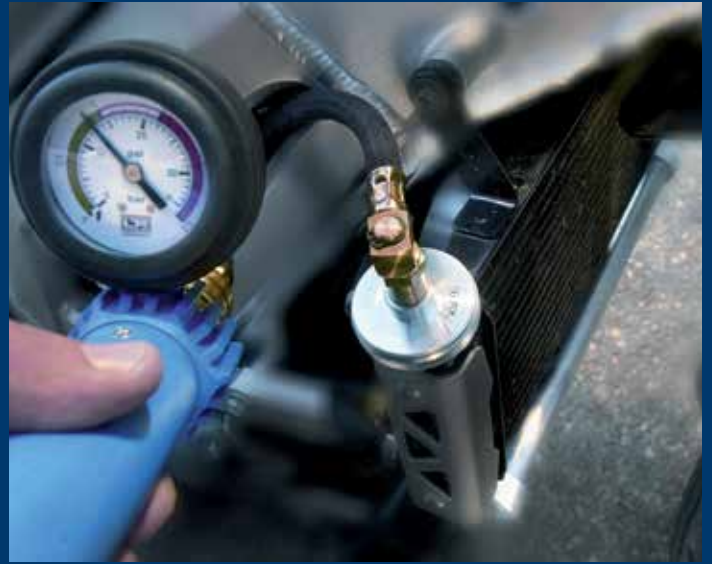
Pump for generating pressure
