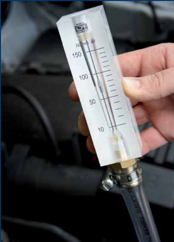
Blow-by-gases measurement with the DFL.
