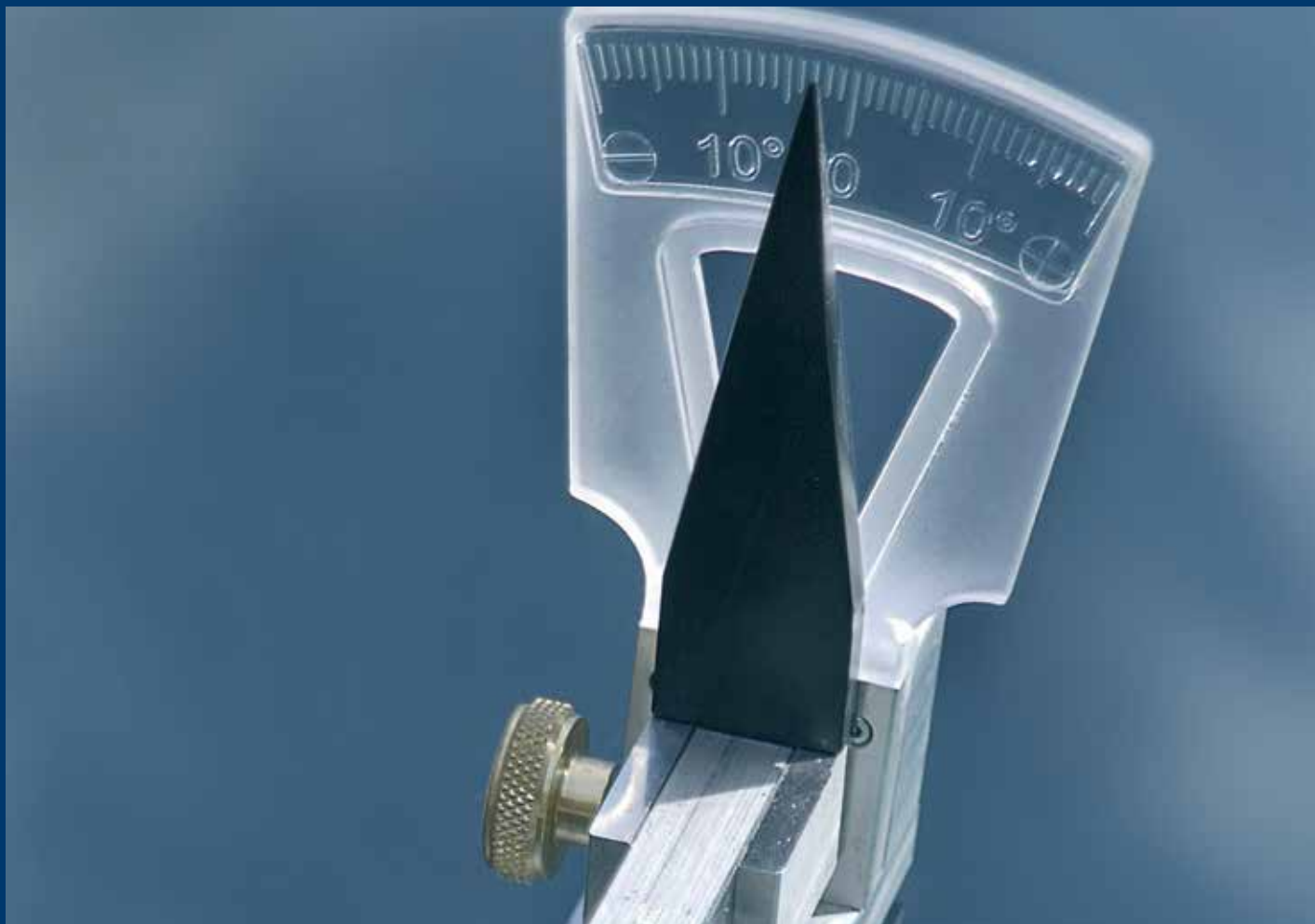
Angle measurement unit for aero wiper testing and adjusting tool
